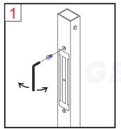
Use 3 mm hexagon tool wrench Use 4 mm hexagonal screw to operate the screw.
